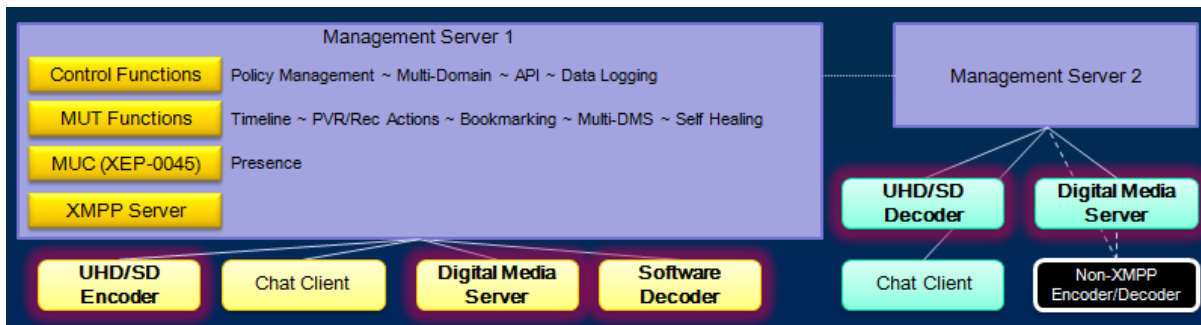
Figure 3. XMPP MUT and Control Layer Architecture and Benefits
